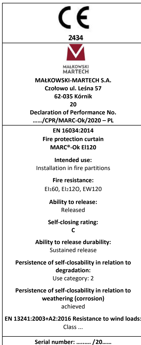
Fig. 13 – Specimen of the nameplate of the fire protection curtain (ref. EN 16034:2014-11)
